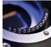
(Above) Close-up of the lens mount (Left) Connectors at the back of the
